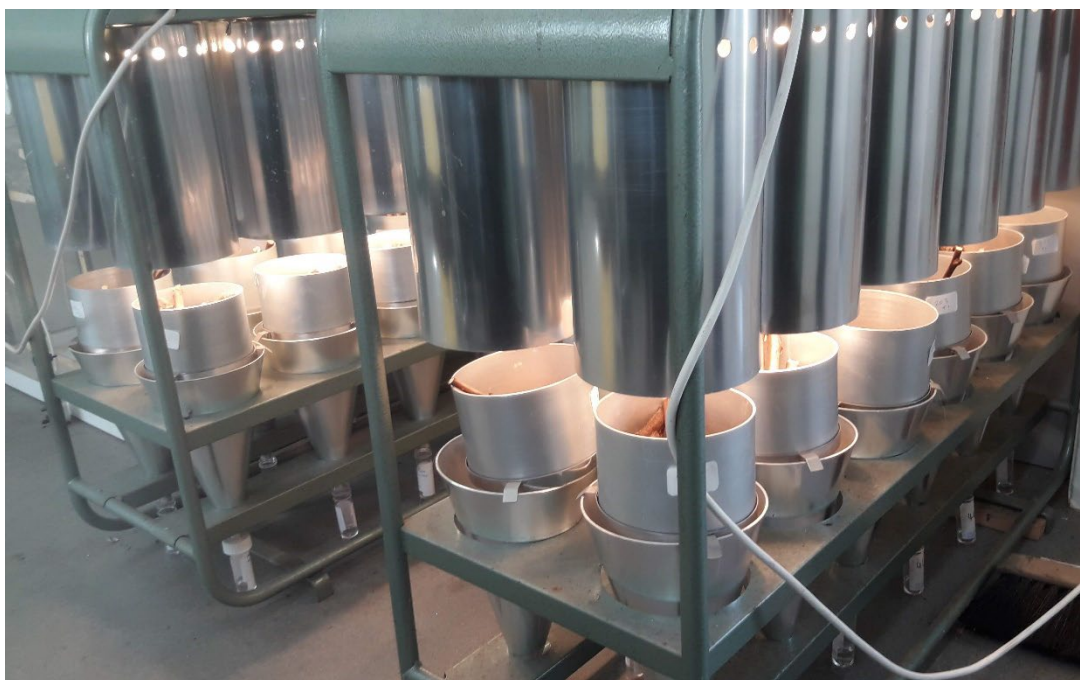
Figure 2.9 Tullgren Funnels containing raspberry cane material. Heat and light from the bulb causes mites in the canes to move downwards through the sieve and into a collecting tube.
